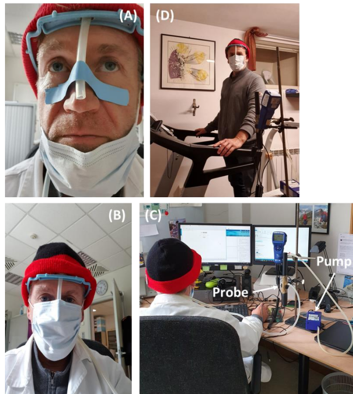
Fig. 1. Experimental setup. (A) Sampling point close to the nose tip; (B) Position of the sampling point while the face mask was worn; (C) Activity pattern 'Office work'; (D) Activity pattern slow and medium speed walking on a treadmill.
